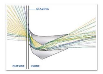
The patented LightLouver reflective slat design redirects all sunlight above a 5 degree altitude angle upward onto the ceiling of the daylit space, providing ambient lighting and eliminating direct sunlight on work surfaces. LightLouver units are a perfect solution for East, West and South facing windows.
